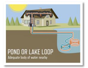
Pond or lake loops are economical to install. Coils of pipe are simply placed on the bottom of the pond or lake.
