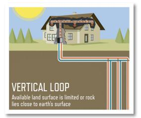
Vertical loops use drilling equipment to bore small-diameter holes from 50 to 200 feet deep. Piping is then fed down these holes creating a loop pattern. The individual loops are all joined together and tied to the indoor heat pump unit.
